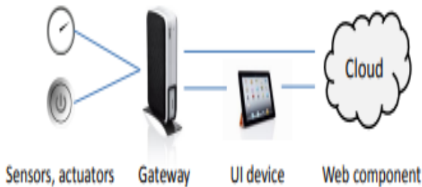
Fig. 2. The Components of an IoT Application (Mazhelis and Tyrväinen, 2014).
